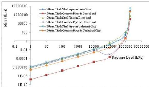
Figure 18: Invert misis of varying pressure load for coefficient of friction of 0.3 in explosion above the ground surface for "No Slip" at the period of 0.025 ms
