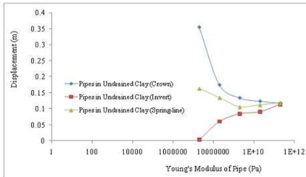
Figure 14: Displacement of varying Young's Modulus of pipe for coefficient of friction of 0.3 in explosion above the ground surface for 'No Slip' and Load intensity of 2000000Pa at the period of 0.025 ms
