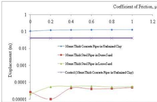
Figure 2: Invert displacement for varying coefficient of friction in explosion above the ground surface with 'No Slip' as control
