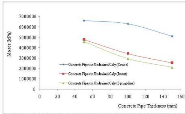
Figure 8: Mises of concrete pipes for coefficient of friction of 0.3 in explosion above the ground surface
