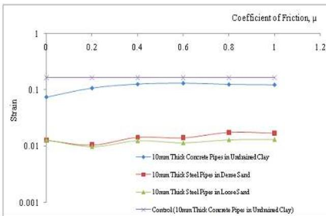
Figure 6: Crown strain for varying coefficient of friction in explosion above the ground surface with 'No Slip' as control
