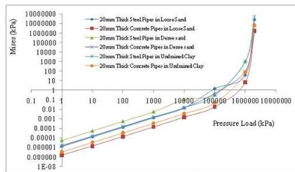
Figure 17: Crown misis of varying pressure load for coefficient of friction of 0.3 in explosion above the ground surface for "No Slip" at the period of 0.025 ms
