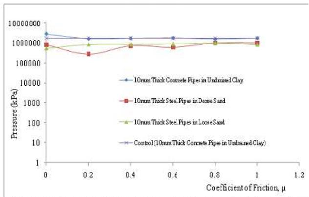
Figure 3: Spring-line pressure for varying coefficient of friction in explosion above the ground surface with 'No Slip' as control
