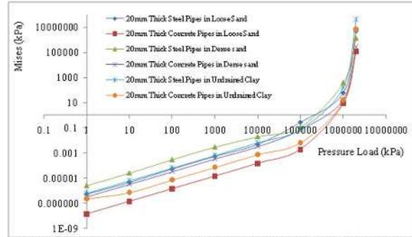
Figure 19: Spring-line misis of varying pressure load for coefficient of friction of 0.3 in explosion above the ground surface for "No Slip" at the period of 0.025 ms
