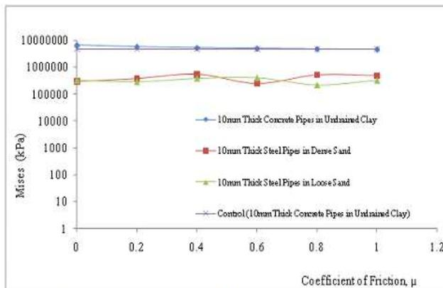
Figure 4: Invert mises for varying coefficient of friction in explosion above the ground surface with 'No Slip' as control
