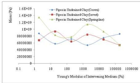
Figure 16: Strain of varying Young's Modulus of intervening medium for coefficient of friction of 0.3 in explosion above the ground surface for "No Slip" and Load intensity of 2000000Pa at the period of 0.025 ms
