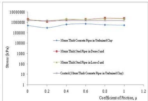
Figure 5: Crown stress for varying coefficient of friction in explosion above the ground surface with 'No Slip' as control
