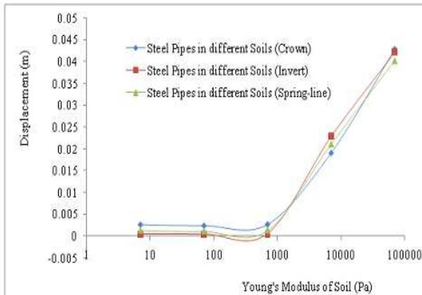
Figure 12: Displacement of varying Young's Modulus of soil for coefficient of friction of 0.3 in explosion above the ground surface for 'No Slip' and Load intensity of 2000000Pa at the period of 0.025 ms
