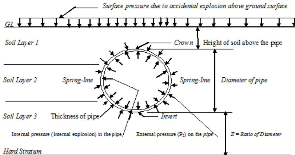
Figure 1: Cross-section of pipe in different soil layers (Olaewaju et al., 2012; Olaewaju, 2013; Olaewaju, 2015; ABAQUS Analysis User’s Manuals. 2009; ABAQUS/Explicit: Advanced Topics, 2009; Geotechnical Modeling and Analysis with ABAQUS, 2009)
