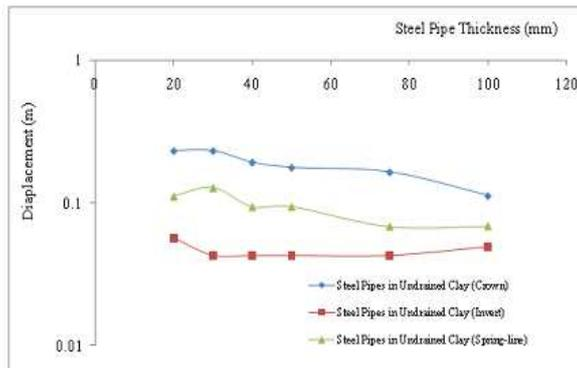
Figure 10: Displacement of steel pipes for coefficient of friction of 0.3 in explosion above the ground surface
