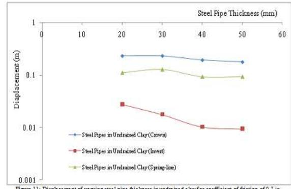
Figure 11: Displacement of varying steel pipe thickness in undrained clay for coefficient of friction of 0.3 in explosion above the ground surface
