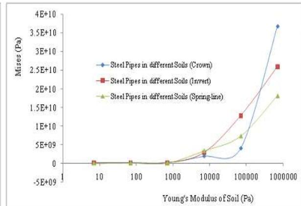
Figure 13: Mises of varying Young's Modulus of soil for coefficient of friction of 0.3 in explosion above the ground surface for 'No Slip' and Load intensity of 2000000Pa at the period of 0.025 ms
