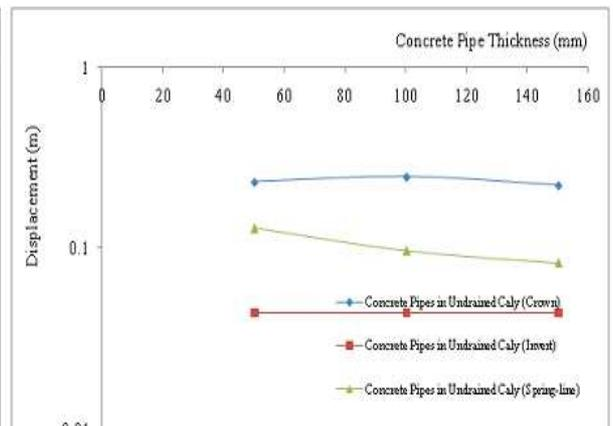
Figure 7: Displacement of concrete pipes for coefficient of friction of 0.3 in explosion above the ground surface
