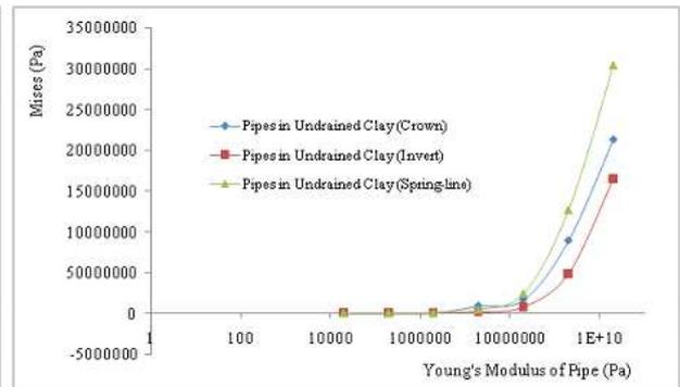
Figure 15: Mises of varying Young's Modulus of pipe for coefficient of friction of 0.3 in explosion above the ground surface for 'No Slip' and Load intensity of 2000000Pa at the period of 0.025 ms
