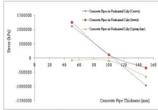
Figure 9: Stress of concrete pipes for coefficient of friction of 0.3 in explosion above the ground surface
