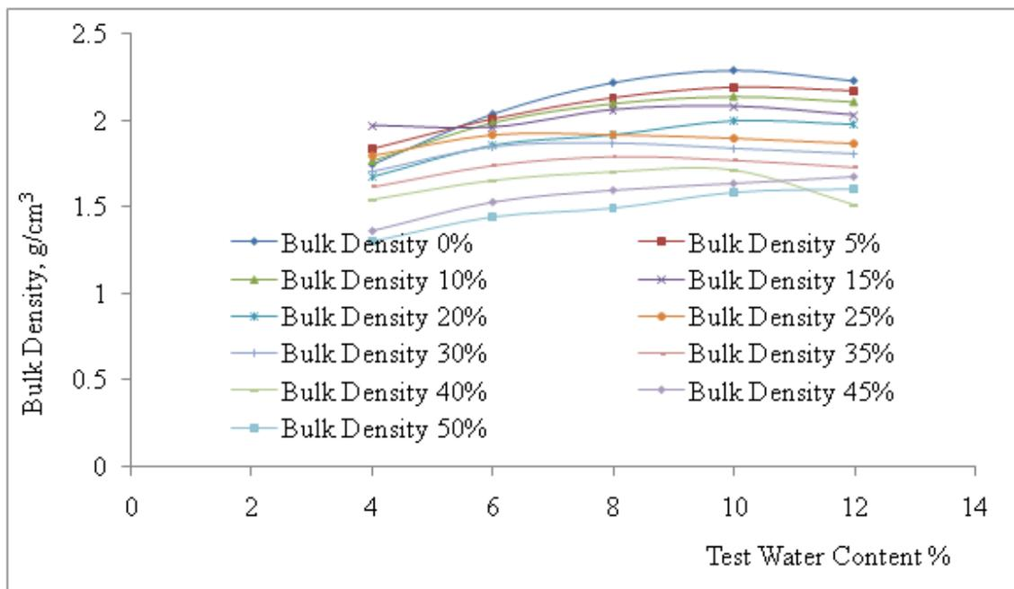
Figure 2: Bulk density against test water content for varying degrees of plastic pellet substitution in lateritic soil
