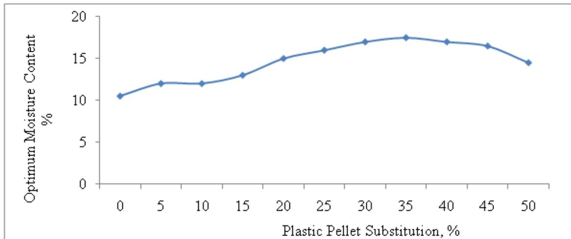
Figure 5: Optimum moisture content against plastic pellet substitutions
