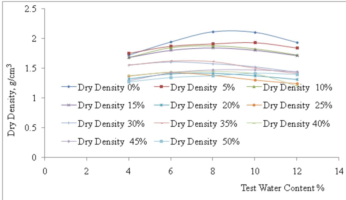
Figure 3: Dry density against test water content for varying degrees of plastic pellet substitution in lateritic soil
