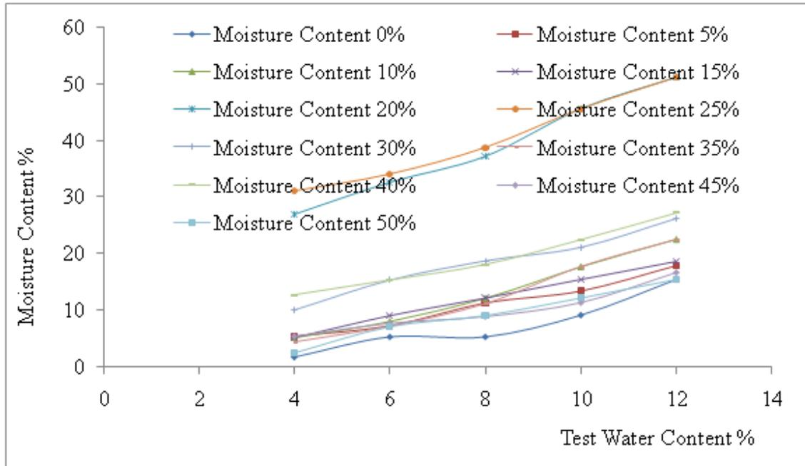
Figure 1: Moisture content against test water content for varying degrees of plastic pellet substitution in lateritic soil
