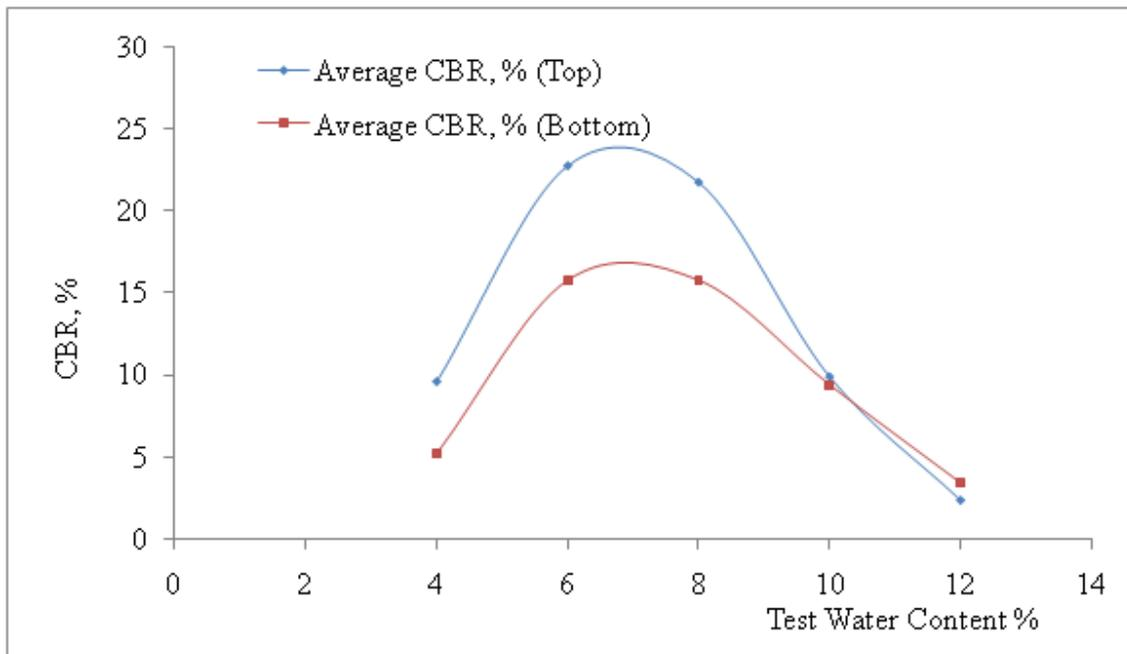
Figure 5: Results of CBR for top and bottom against test moisture content for 15% palm kernel shell substitution in lateritic soil
