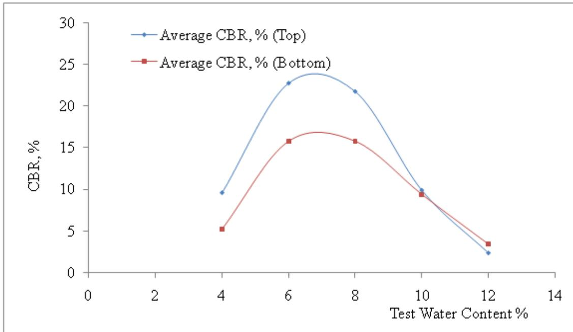
Figure 6: Results of CBR for top and bottom against test moisture content for 20% palm kernel shell substitution in lateritic soil
