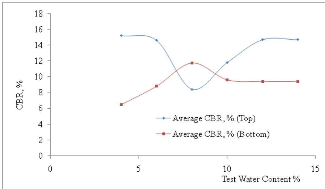
Figure 12: Results of CBR for top and bottom against test moisture content for 50% palm kernel shell substitution in lateritic soil
