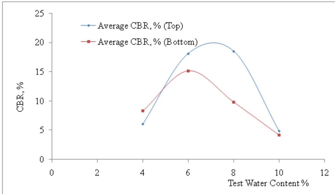
Figure 2: Results of CBR for top and bottom against test moisture content for 0% palm kernel shell substitution in lateritic soil (control experiment)
