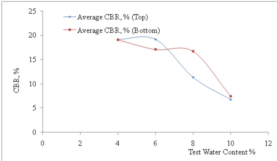
Figure 10: Results of CBR for top and bottom against test moisture content for 40% palm kernel shell substitution in lateritic soil
