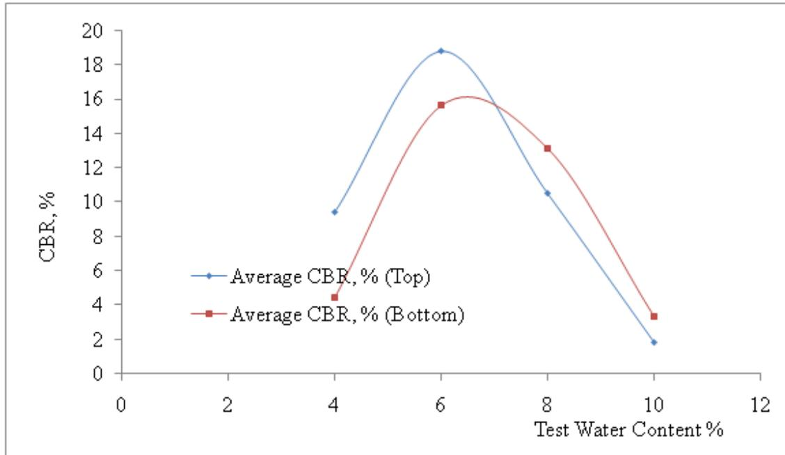
Figure 3: Results of CBR for top and bottom against test moisture content for 5% palm kernel shell substitution in lateritic soil
