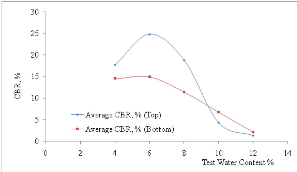
Figure 4: Results of CBR for top and bottom against test moisture content for 10% palm kernel shell substitution in lateritic soil
