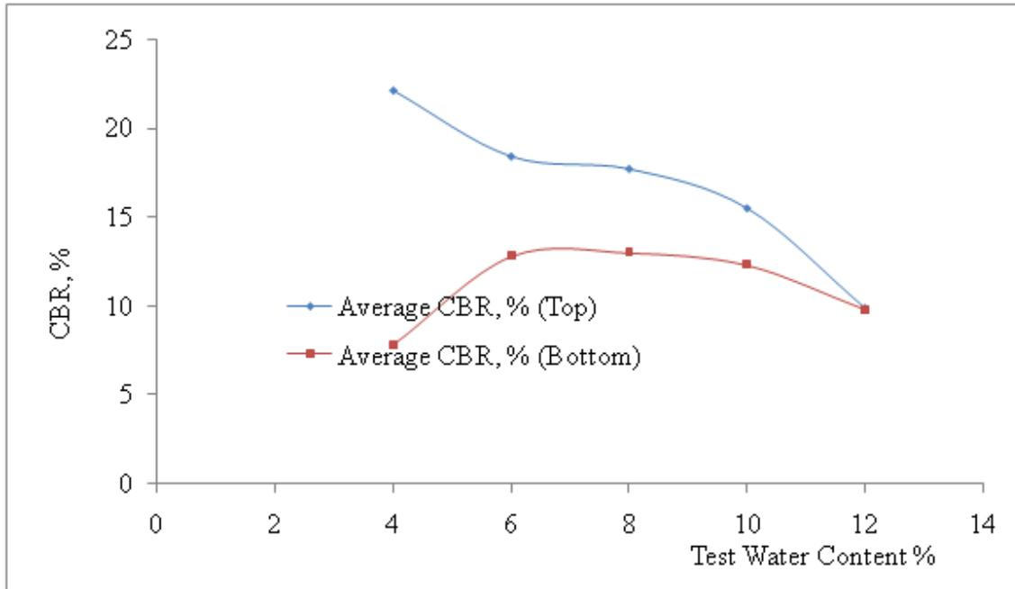
Figure 11: Results of CBR for top and bottom against test moisture content for 45% palm kernel shell substitution in lateritic soil
