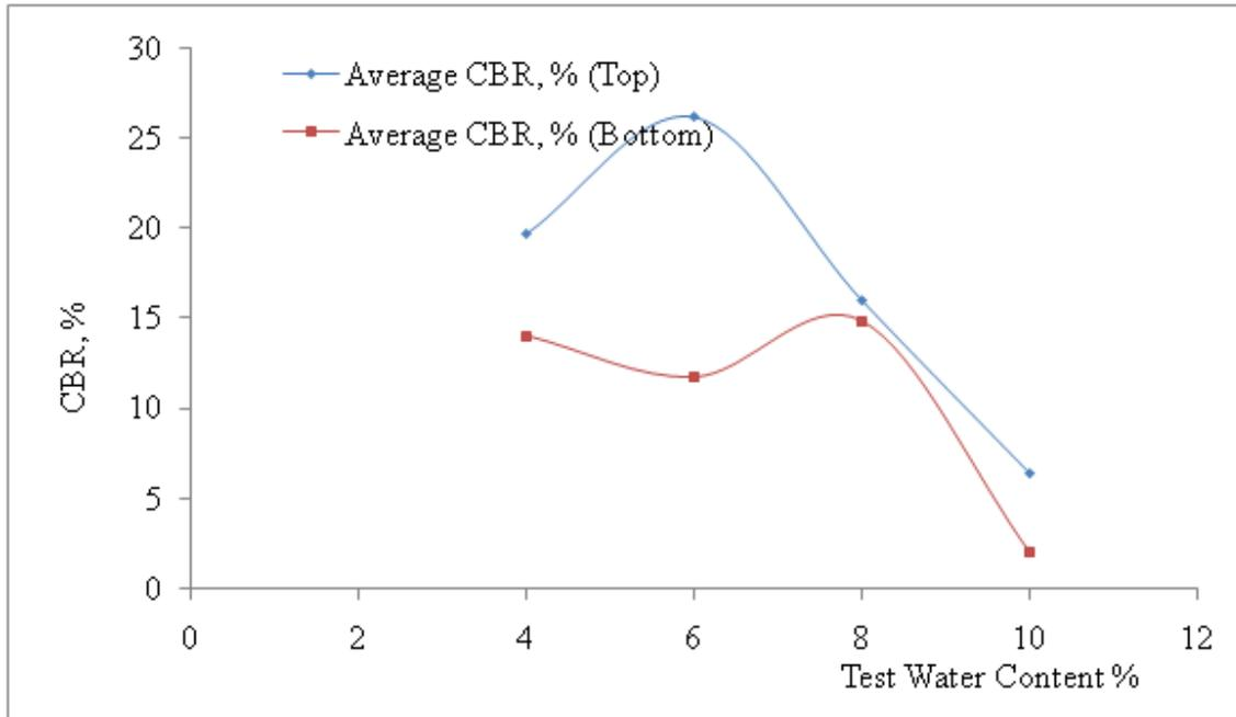
Figure 9: Results of CBR for top and bottom against test moisture content for 35% palm kernel shell substitution in lateritic soil
