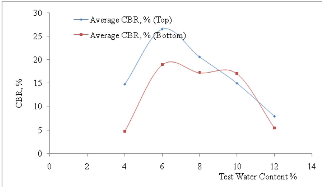
Figure 8: Results of CBR for top and bottom against test moisture content for 30% palm kernel shell substitution in lateritic soil
