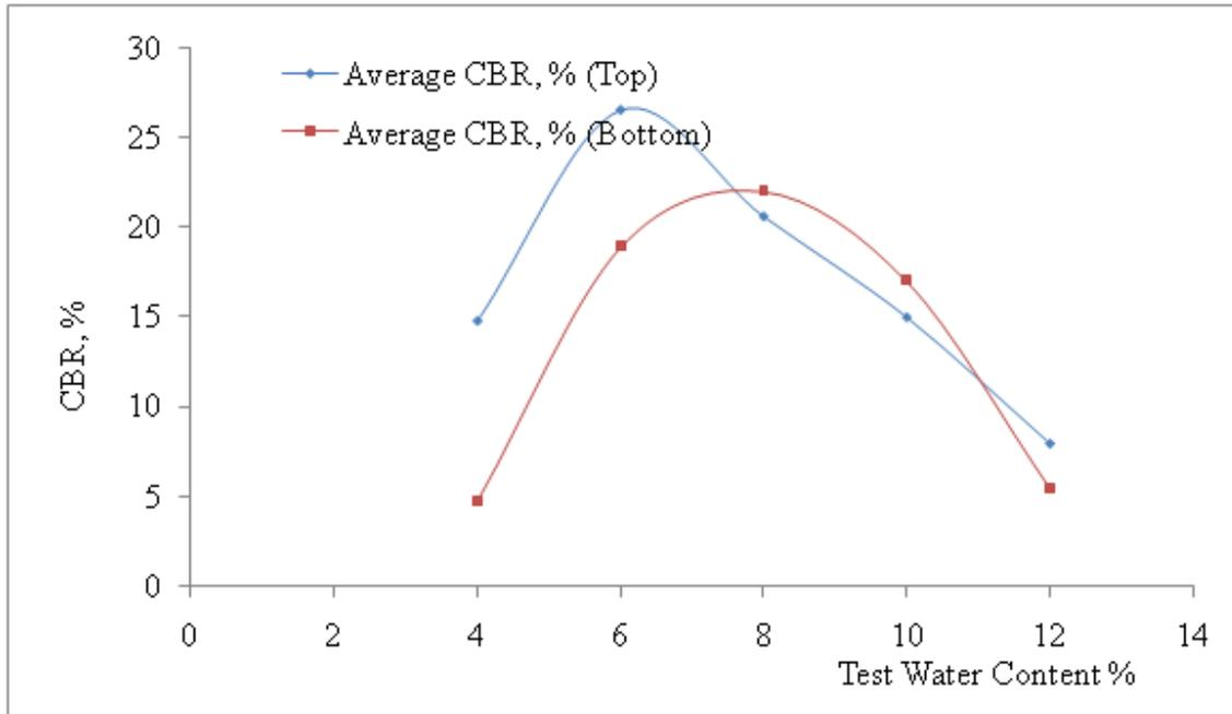
Figure 7: Results of CBR for top and bottom against test moisture content for 25% palm kernel shell substitution in lateritic soil
