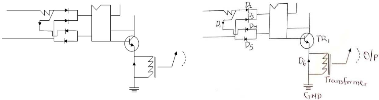
Figure 2: The changeover circuit of the UPS
