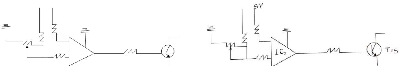
Figure 3: Low battery cut off
