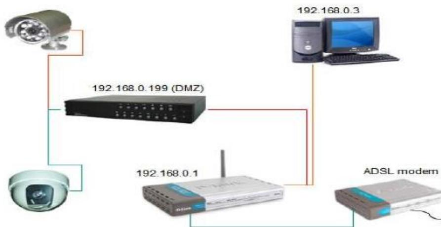
Figure 2: The proposed Video Surveillance System using IP-based CCTV cameras
