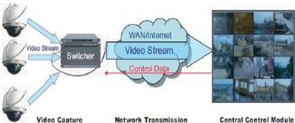
Figure 1: A typical video surveillance camera control system
