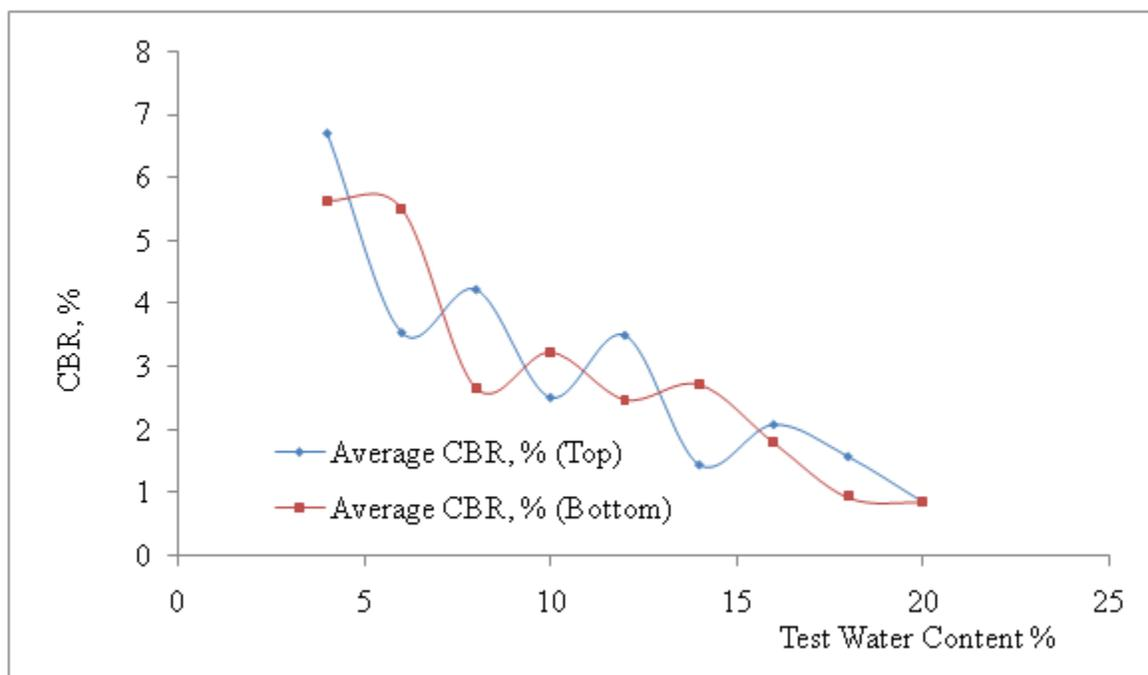
Figure 11: Results of average CBR for top and bottom against test water content in black cotton soil on basement complex
