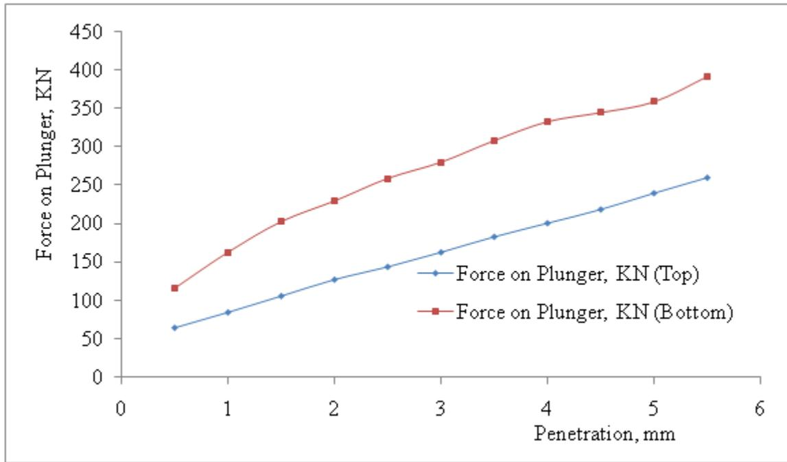
Figure 4: Results of force on plunger for top and bottom against penetration for 8% moisture content in black cotton soil on basement complex
