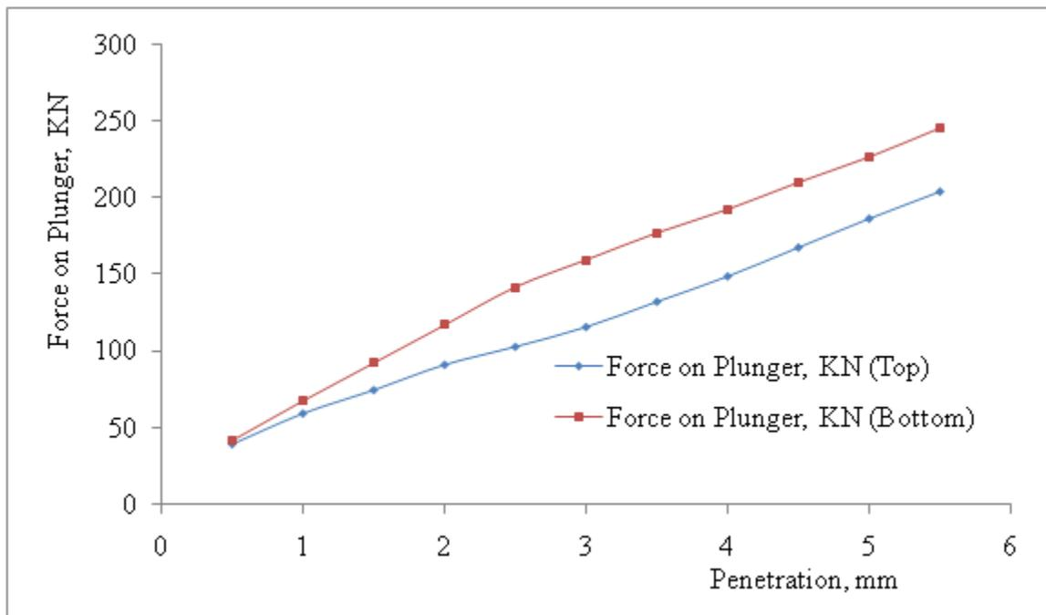
Figure 5: Results of force on plunger for top and bottom against penetration for 10% moisture content in black cotton soil on basement complex
