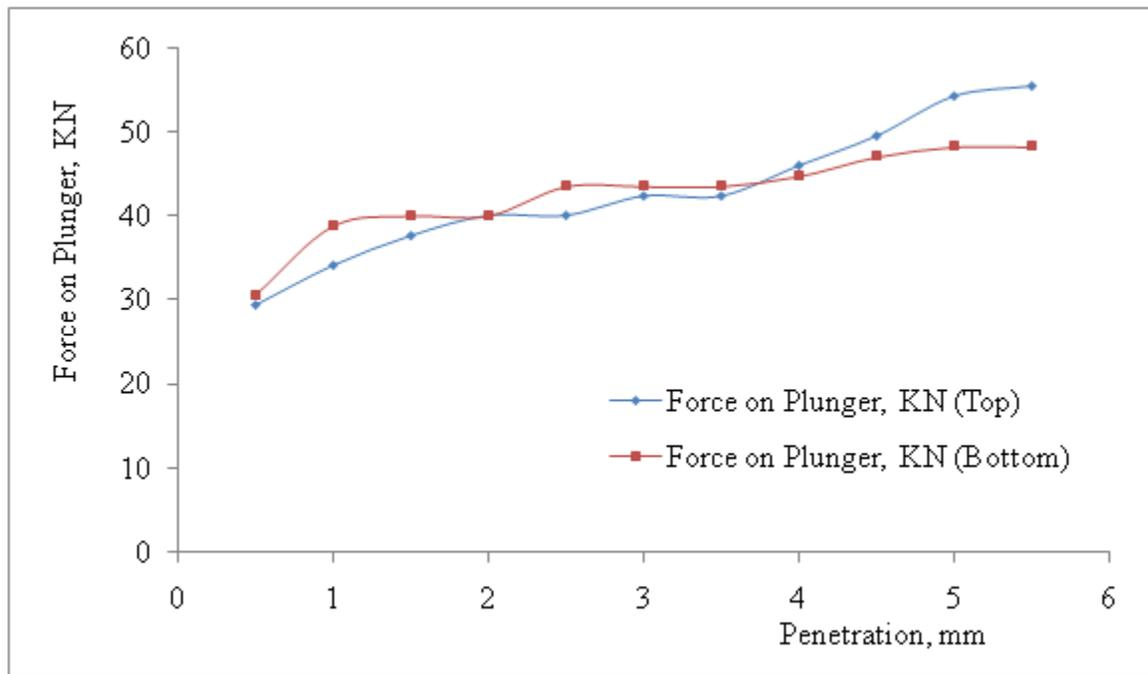
Figure 10: Results of force on plunger for top and bottom against penetration for 20% moisture content in black cotton soil on basement complex
