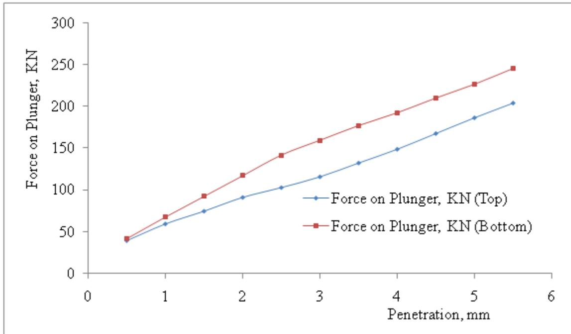
Figure 6: Results of force on plunger for top and bottom against penetration for 12% moisture content in black cotton soil on basement complex
