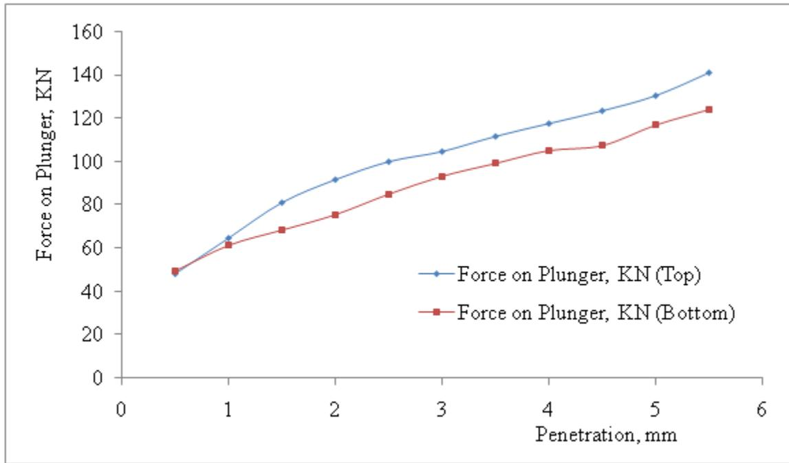
Figure 8: Results of force on plunger for top and bottom against penetration for 16% moisture content in black cotton soil on basement complex
