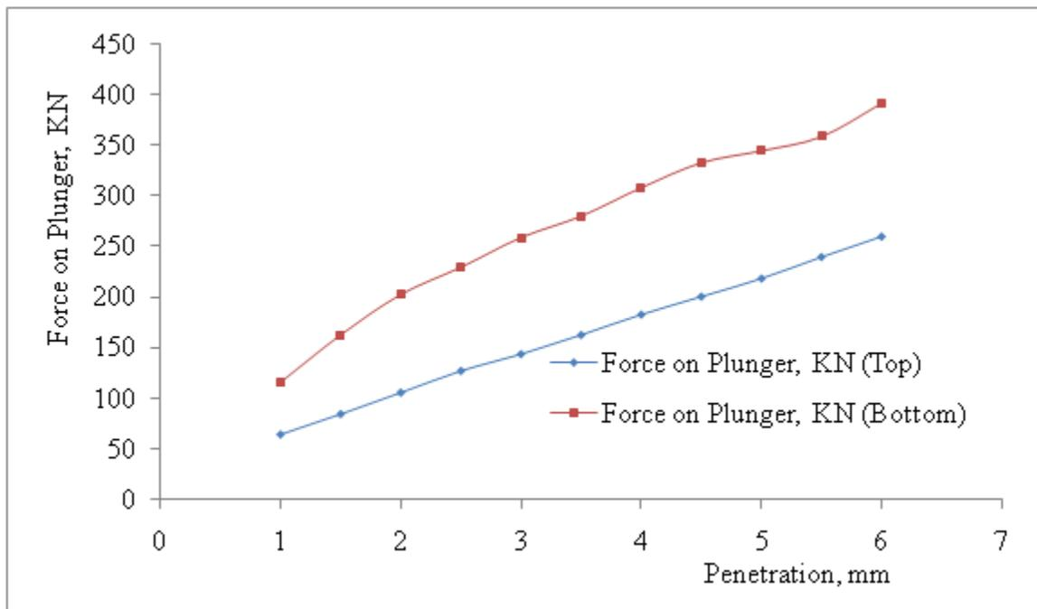
Figure 3: Results of force on plunger for top and bottom against penetration for 6% moisture content in black cotton soil on basement complex
