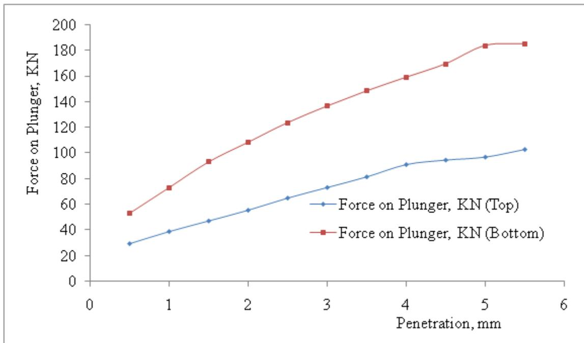
Figure 7: Results of force on plunger for top and bottom against penetration for 14% moisture content in black cotton soil on basement complex
