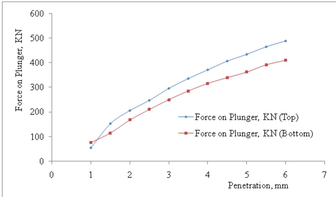
Figure 2: Results of force on plunger for top and bottom against penetration for 4% moisture content in black cotton soil on basement complex
