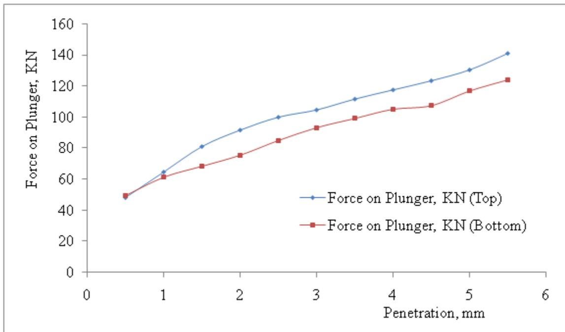
Figure 9: Results of force on plunger for top and bottom against penetration for 18% moisture content in black cotton soil on basement complex
