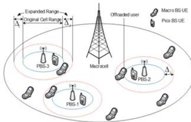
Fig. 1: Cell selection with range expansion in HetNet
