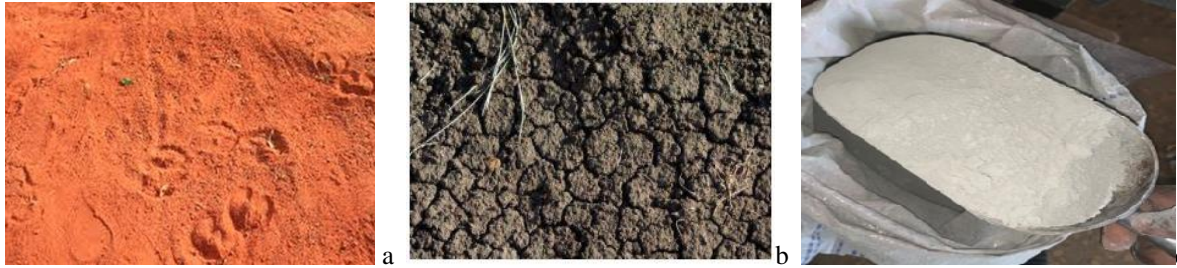
Figure 1: a Lateritic soil, b Black Cotton Soil and c Ordinary Portland Cement
