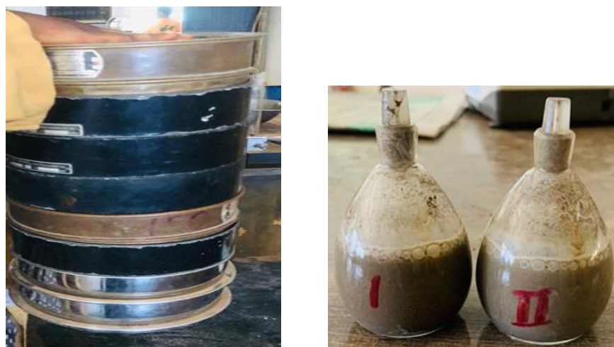
Figure 2: a. Sieve sizes distribution, b. Specific Gravity using Pycnometers
